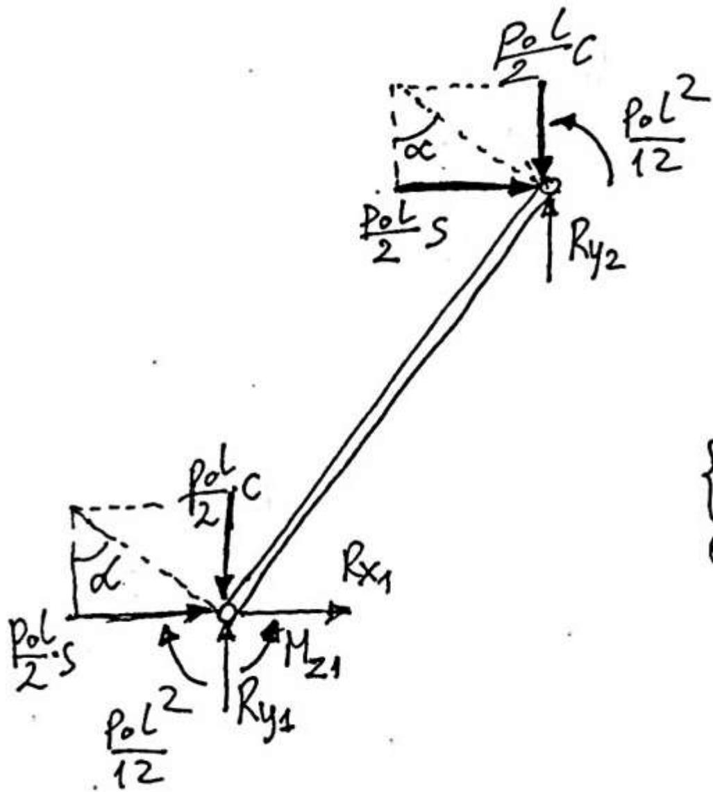
$$\{F\}_{6 \times 1} = \left\{ \begin{array}{l} R_{x_1} + \frac{P_{oL}}{2} \cdot S \\ R_{y_1} - \frac{P_{oL}}{2} \cdot C \\ M_{z_1} - \frac{P_{oL}^2}{12} \\ \frac{P_{oL}}{2} \\ R_{y_2} - \frac{P_{oL}}{2} \cdot C \\ \frac{P_{oL}^2}{12} \end{array} \right\}$$
