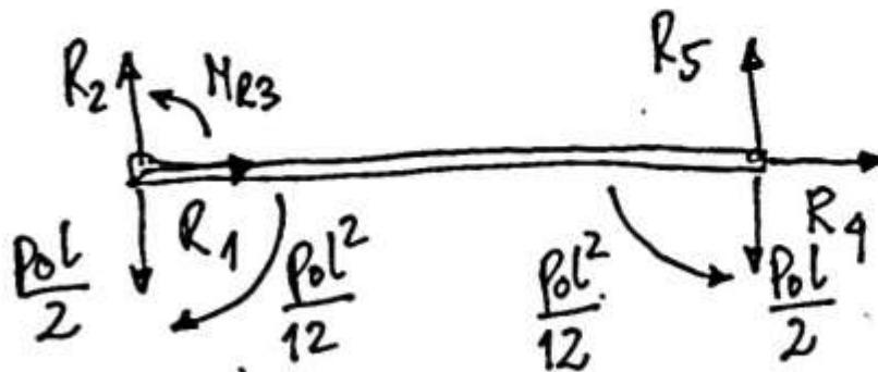
$$\{F\}_{6 \times 1} = \begin{Bmatrix} R_1 \\ R_2 - \frac{P_o L}{2} \\ M_{R3} - \frac{P_o L^2}{12} \\ R_4 \\ R_5 - \frac{P_o L}{2} \\ \frac{P_o L^2}{12} \end{Bmatrix}$$
